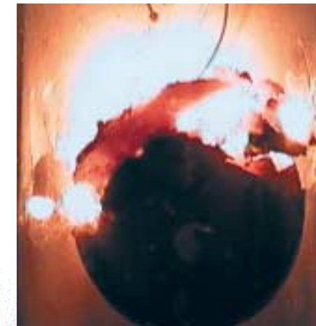
Above: Fireworks in action: a ferrite disc reaches 2000°C in 30 seconds.
